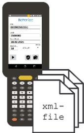
The module BetterPack serves to activate the actual circulated serial numbers. The data matrix codes of the packed folding boxes will be scanned, so that their serial numbers can be stored in a xml-file which can be uploaded in the verification system. The generated xml-files of the BetterPack application can either be uploaded manually in the national verification system or the European Hub. Alternatively, the data transmission can be integrated in the BetterPack application.
